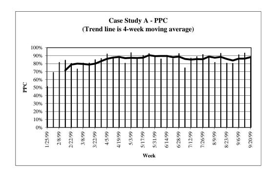
Productivity was not measured on this project; the only metric measured by site management was PPC. By Lean Construction theory, productivity factors are considered in developing the weekly work plans, so that if all assignments on the weekly work plan are completed, the incorporated productivity factor is met by design. The collection, analysis, and comparison of PPC and productivity data on the same project would provide an interesting comparison.
